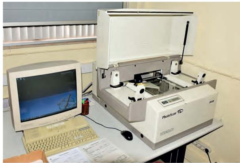
Figura 7 - Scanner fotogramétrico ( PhotoScan TD, Intergraph )
