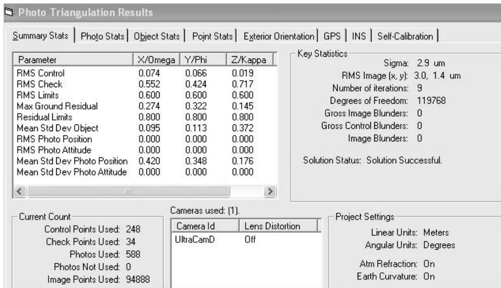
Figure 4 - Aerotriangulation results.
