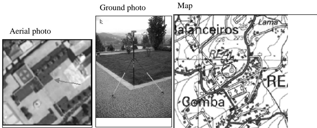
Figure 3 - Example of a photogrammetric point of Oporto block.
